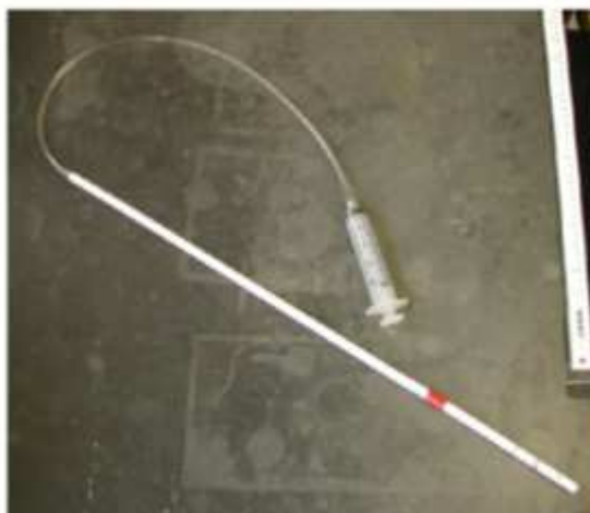
Figure 5.3. Soil sipper consisting of a syringe, flexible plastic tubing, and rigid plastic tubing.
